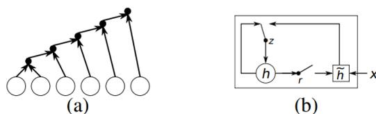
**Figure 1:** The graphical illustration<sup>22</sup> of (a) the recurrent neural network and (b) the hidden unit of GRU that adaptively forgets and remembers.
