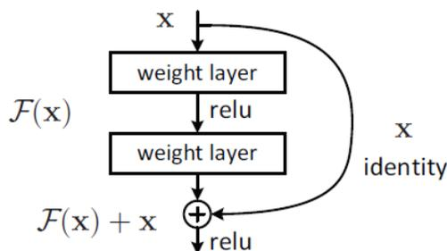
**Figure 2:** A Residual Learning Block<sup>12</sup>. Compared with a traditional multi-layer perceptron, the change is that some layers that used to be non-adjacent are connected.
