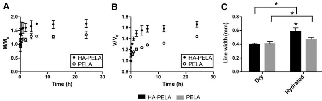
**FIG. 3.** Swelling behavior of HA-PELA and PELA scaffolds ( $n=3$ ). (A) Change in scaffold mass (swelled mass  $[M]$ /initial mass  $[M_0]$ ) over time in deionized water at 37°C. (B) Change in scaffold volume (swelled volume  $[V]$ /initial volume  $[V_0]$ ) over time in deionized water at 37°C. (C) Change in line width after 24 h hydration in deionized water at 37°C ( $*p < 0.05$ ).
