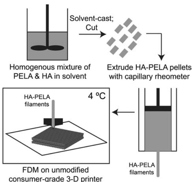
**FIG. 1.** Depiction of the preparation of PELA and HA-PELA three-dimensional (3D) scaffolds by rapid prototyping. HA, hydroxyapatite, PELA, poly(D,L-lactic acid)-poly(ethylene glycol)-poly(D,L-lactic acid).
