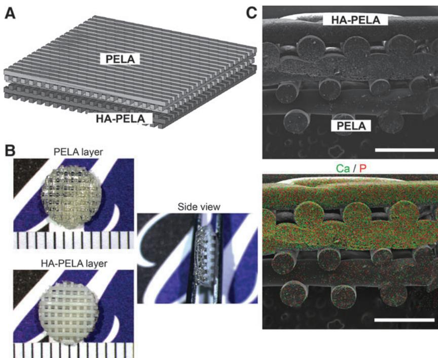
**FIG. 8.** PELA/HA-PELA biphasic scaffold. **(A)** CAD model of the PELA/HA-PELA biphasic scaffold. **(B)** Stereomicroscopy images of a 6-mm core punched out from the biphasic scaffold. Scale markings = 1.0 mm **(C)** Scanning electron micrograph of a biphasic scaffold (*top*). Elemental mapping overlay (*bottom*) of calcium (*green*) and phosphate (*red*). Scale bars = 1 mm. Color images available online at [www.liebertpub.com/tec](http://www.liebertpub.com/tec)
