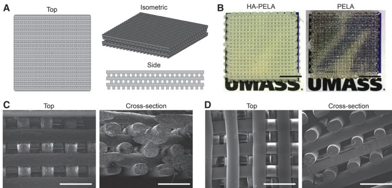
**FIG. 2.** (A) Top, isometric, and side views of scaffold CAD design. (B) Stereomicroscopy images of rapid prototyped HA-PELA and PELA scaffolds. Scale bars = 5 mm. (C) Scanning electron micrographs of the HA-PELA scaffold. Scale bars = 1 mm. (D) Scanning electron micrographs of the PELA scaffold. Scale bars = 1 mm. Color images available online at [www.liebertpub.com/tec](http://www.liebertpub.com/tec)
