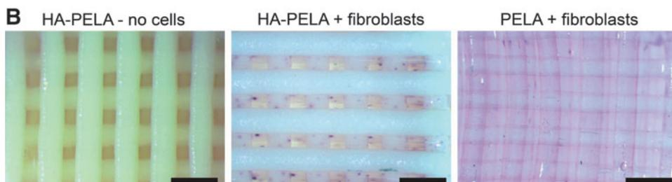
**FIG. 6.** (A) CCK-8 cell viability assay of NIH3T3 attachment and proliferation on HA-PELA and PELA scaffolds ( $n=3$ ) ( $*p < 0.05$ ). (B) Stereomicroscopy images of MTT stained scaffolds 24 h post-NIH3T3 seeding. Dark purple stains denote viable cells adhered on the scaffolds. Scale bars = 1 mm. Color images available online at [www.liebertpub.com/tec](http://www.liebertpub.com/tec)
