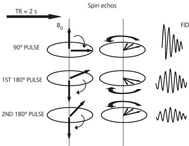
FIG. 4. Schematic diagram showing the behaviour of precessing hydrogen nuclei in a spin echo pulse sequence. Net magnetisation (red arrows) in the main magnetic field ( $B_0$ ) slowly relaxes back to equilibrium over successive  $180^\circ$  pulses following the initial  $90^\circ$  pulse. Time to repeat (TR) is the repetition time between  $90^\circ$  pulses (31).
