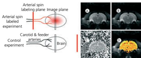
FIG. 7. Schematic diagram showing arterial spin labelling procedure and image processing. (A) Control image. (B) Image acquired with arterial spin labelling. (C) Label/Control – 1. (D) False coloured overlay of blood flow. Note the enhanced blood flow to the cortex as compared to subcortical areas. Legend scale 0 ± 12%.
