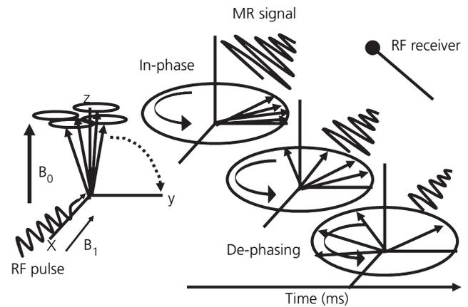
FIG. 3. Schematic diagram showing behaviour of hydrogen nuclei flipped into the transverse x-y plane with a radiofrequency (RF) pulse.  $B_0$  is the main magnetic field and  $B_1$  is the magnetic field created in the transverse plane by the RF pulse (31).
