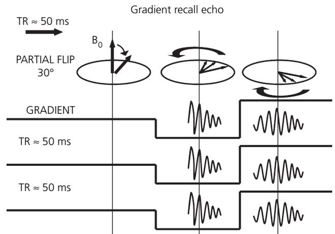
FIG. 6. Schematic diagram showing the behaviour of precessing hydrogen nuclei partially flipped into the transverse plane at an angle of  $30^\circ$ . During the short-lived event, the gradient coils are used to reverse the magnetic field (black horizontal line) to refocus the precessing nuclei (31). TR, Time to repeat.
