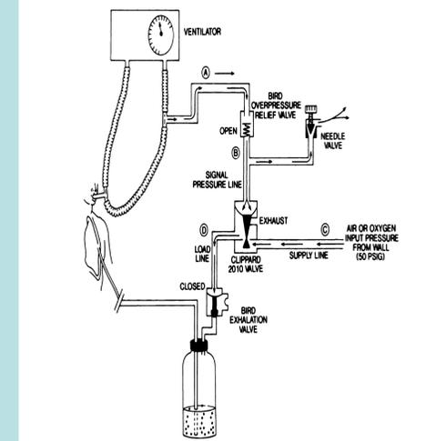
Figure 2. During the exhalation phase, airway pressure decreases which causes the overpressure relief valve to close. The pressure loading diaphragm (A) in the amplifier valve dissipates via a needle valve, which closes the amplifier valve. Thus, the exhalation valve opens and allows the chest tube and the underwater seal apparatus to function in the normal manner<sup>12</sup>.
