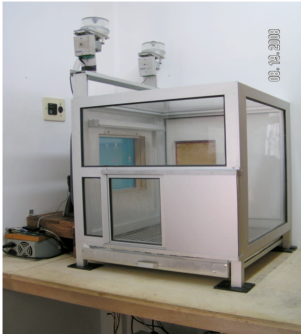
Figure 1. Experimental chamber. The picture shows the sliding door, the touch screen monitor on the left, the pellet receptacles above, and two pellets dispensers externally and above. The door providing access to the outside is on the back wall. A videocamera could be installed externally to the right Plexiglas wall.
